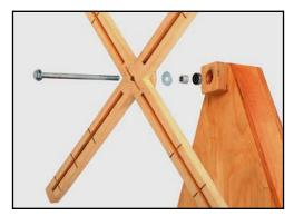
Insert 3/8 x 7" carriage bolt through the hole in the center of the cross arms. Be sure the metal plate and engraved size markings are facing forward. The square neck of the carriage bolt seats in the square hole on the front of the arms.
