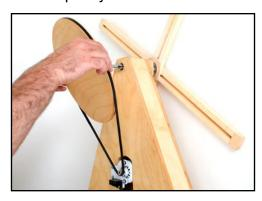
Loop the v-belt around the large wooden pulley and hold with one hand on each
