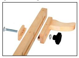
Insert a 5/16 x 2" carriage bolt through the wooden slider pad, so that the square neck of the carriage bolt seats in the square hole in the pad. Hold an adjustable finger on the front of one arm of the cross arms, so that the tongue on the back side of the finger fits in the groove of the arm. Insert the carriage bolt/pad assembly through the back of the arm, and through the hole in the finger, so that the tongue on pad fits into the groove in the arm.
