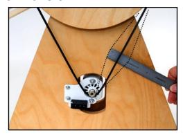
The drive belt tension is adjusted to the correct tension before shipping. However should the motor move during shipping or assembly readjustment may be necessary.
